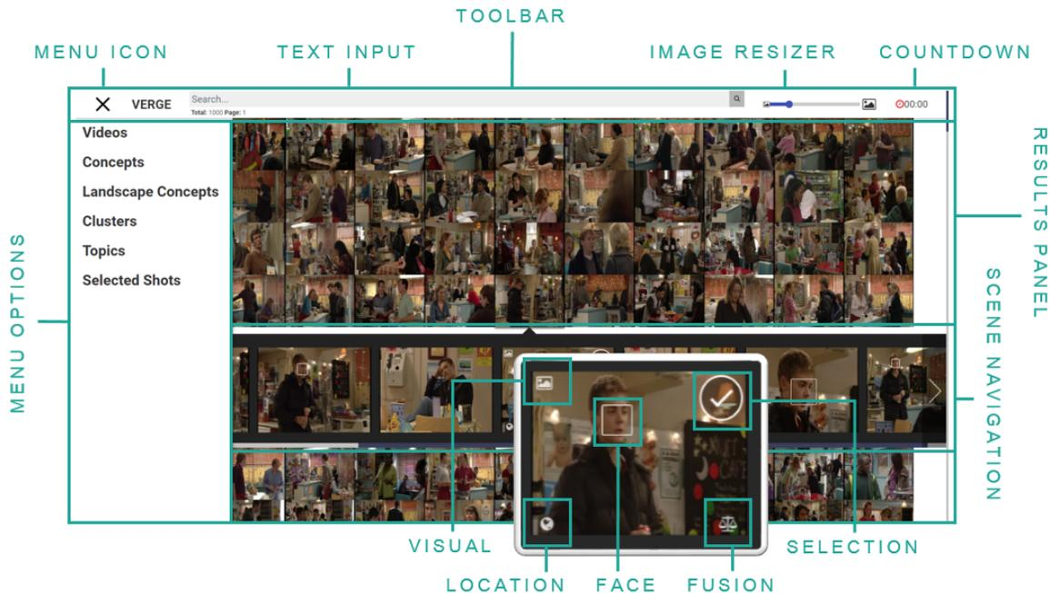
Figure 2: Components of the VERGE application.
