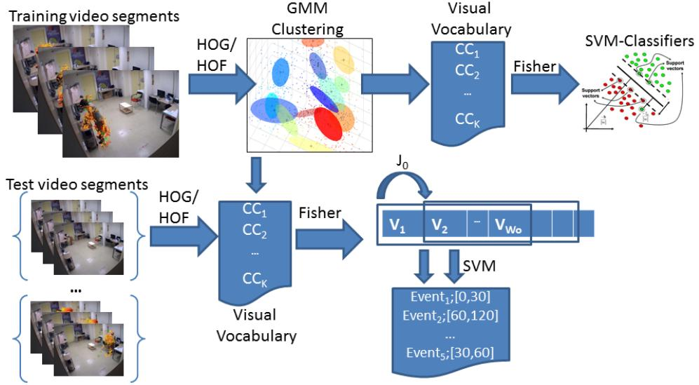
Figure 5: Block diagram of the surveillance event detection system.
