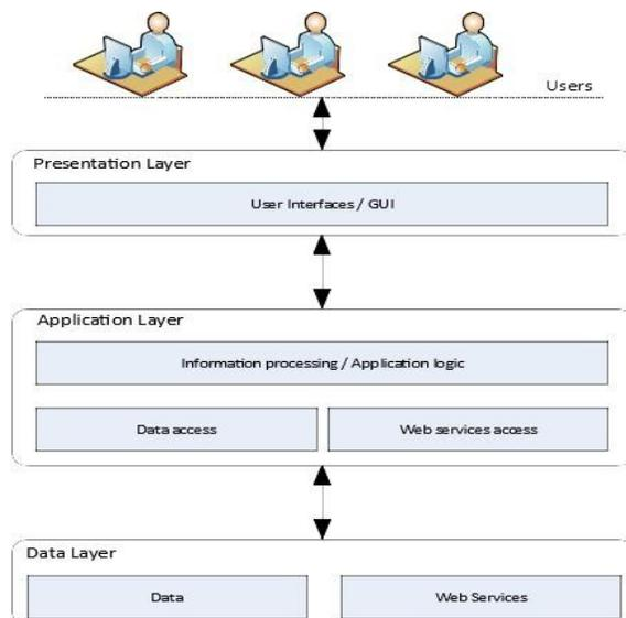
Figure 2: Three-tier Client-Server model.
