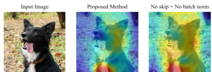
Fig. 5: Qualitative comparison between the proposed attention module and the ‘no skip + no batch norm’ variant, applied to VGG-16. We observe that for the ‘no skip + no batch norm’ architecture, the produced explanation map is more spread out, showing that even if it performs well on the 100% measures, it fails to precisely identify the salient regions in the image.
