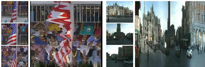
**Fig. 2.** Two tomograph examples, each one corresponding to a different type of tomograph image. The left tomograph is a CH-tomograph, while the right a CV-tomograph. Both of them are defined by the temporal ordering of lines that pass from the center of the frame. Three indicative frames of the shot from which each tomograph was generated are also shown to the left of the corresponding tomograph (the temporal order of the shown frames is from the top to the bottom).
