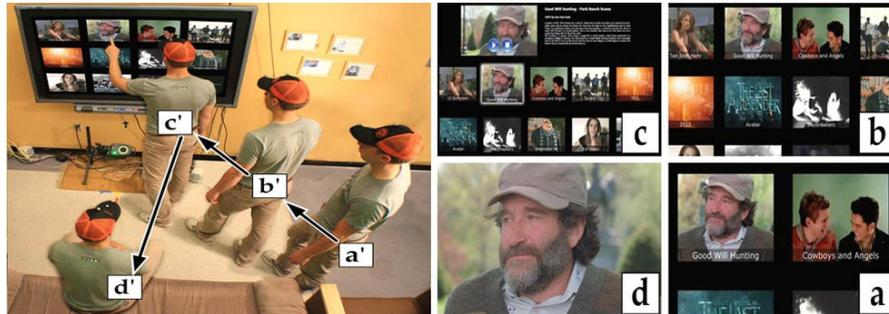
**Fig. 2.** Proxemic Interaction: a) activating the system when a person enters the room, b) continuously revealing of more content with decreasing distance of the person to the display, c) allowing explicit interaction through direct touch when person is in close distance, and d) implicitly switching to full screen view when person is taking a seat. From [23].
