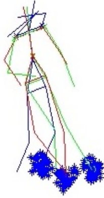
Figure 3: Initialization of candidate positions for left foot (joint id = 12) from three different Kinect Sensors.
