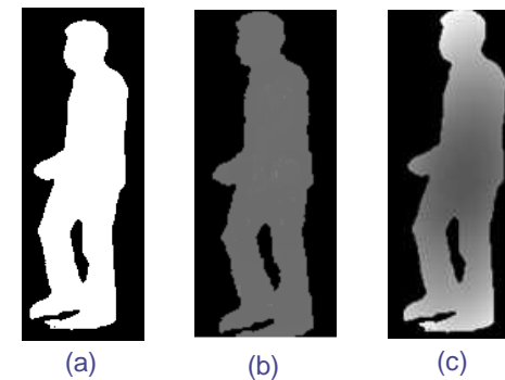
Binary Silhouette (a), 3D Radial Distributed Silhouette (b), and 3D Geodesic Distributed Silhouette (c)
