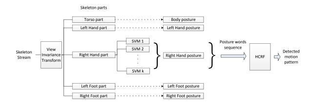
Figure 3: Motion Analysis subsystem
