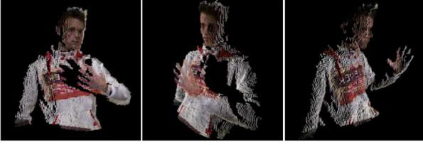
**Fig. 2.** Examples of reconstructed mesh point clouds rendered in 60 FPS running on Google Chrome web browser, a single Kinect, the ZigFu browser plugin and Three.js 3D Library.
