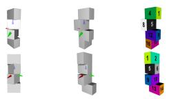
Figure 1: **Left**: The symmetric calibration structure used in [Ale17]. **Middle**: Our asymmetric structure with its corresponding semantic labels per face (**Right**). Instead of aligning the boxes on top of each other using their diagonals, they are now snapping on their top sides' corners, following a  $90^{\circ}$  rotational pattern.
