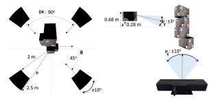
Figure 2: Pose generation process. The range limits of each parameter in equation (1) used to sample/generate the poses are visually presented, showcasing the possible sensor positions around the calibration structure.
