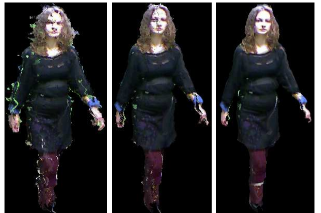
Fig. 5. Xenia: Raw point-set, the output of smoothing operation and the final reconstruction.
