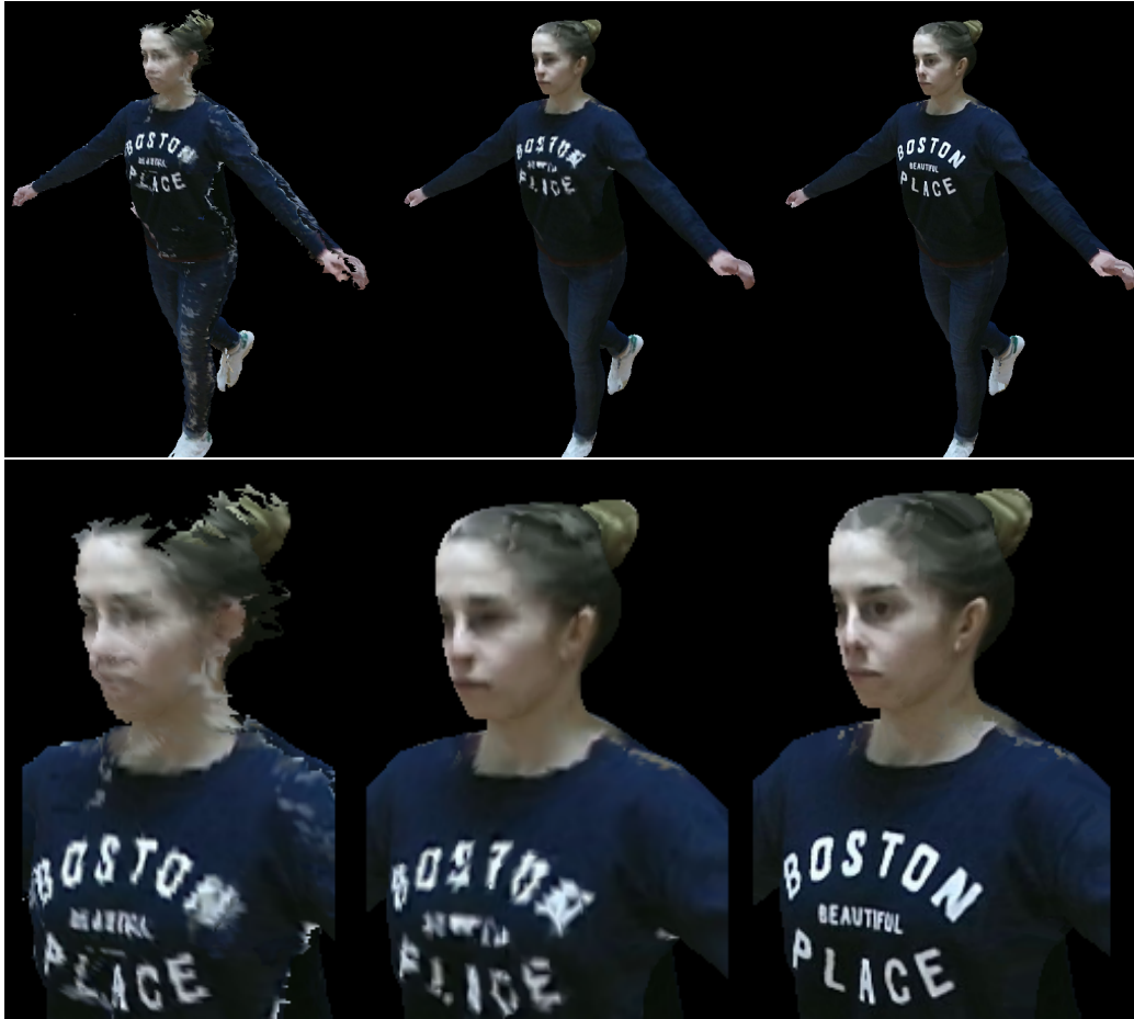
Figure 17: Lenia4 - From left-to-right: (a) Raw textured data; (b) Model-based, color-per-vertex; (c) Model-based with UV texture-mapping for the visible areas. Bottom row: Zoom in the face.
