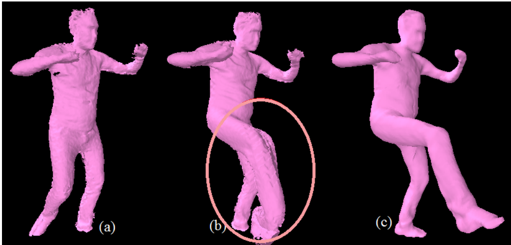
Figure 15: Alexandros - From left-to-right: Reconstruction by (a) a VolumeDeform-like [28] approach at frame t - 5 and (b) at frame t ; (c) by the proposed model-based at frame t . Large motion cannot be efficiently handled by a model-free method, even with the use of RGB-based 2D features, as in [28].
