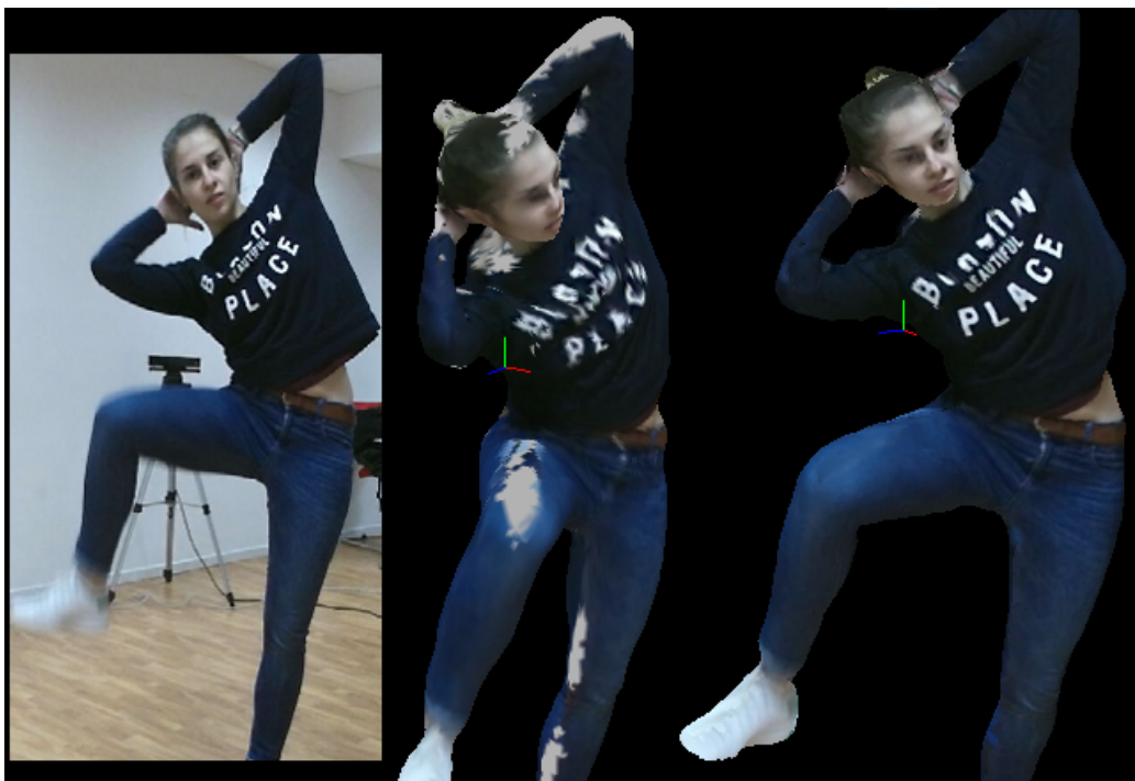
Figure 7: Texturing process. From left to right: i) An original RGB view; ii) Deformed model, with color-per-vertex using the RGB information only in the current frame. Gray vertices are those that are invisible to all cameras; iii) Final rendered model, using color-per-vertex for invisible vertices and UV-texture mapping for the visible ones.
