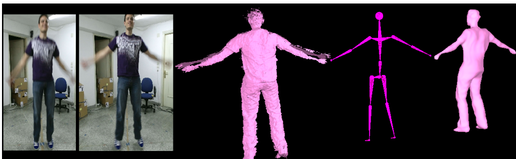
Figure 8: Apostolakis2 sequence - Jumping jacks. Left: Two consecutive frames; Right: The corresponding raw 3D data, the tracked skeleton and the corresponding “puppeted” model, for the 2nd frame.
