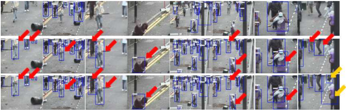
Fig. 2. Example detections on a MET CCTV video trained with ascending levels of blurriness. VOC, VOC5 and VOC10 are depicted in rows 1, 2, 3, respectively. Red arrows depict new detections with VOC5 and yellow new detections with VOC10.
