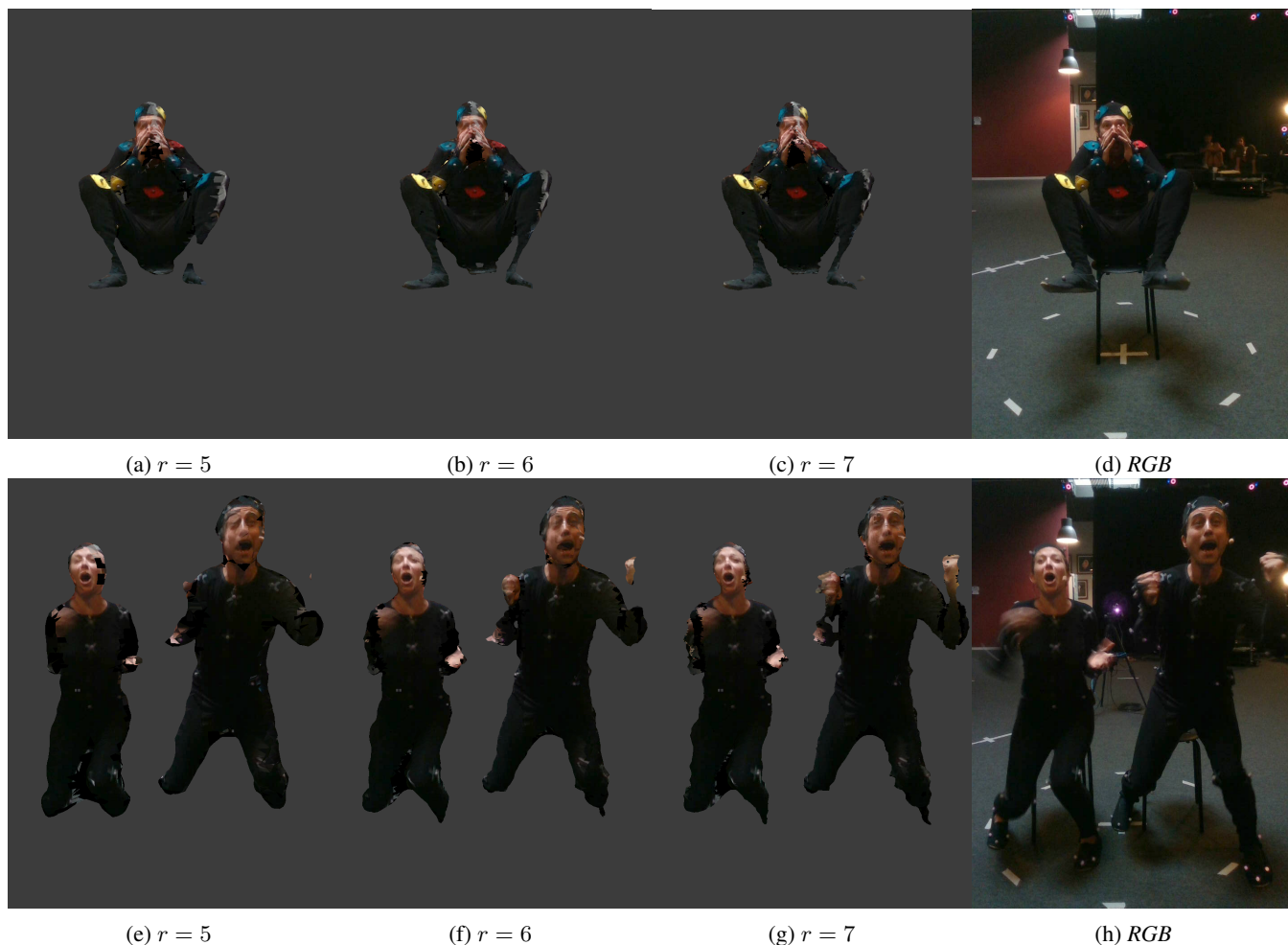
FIGURE 17: Textured mesh-based volumetric samples from H4D1 and H4D2 rendered in the 3 different voxel-grid resolutions along with the corresponding RGB images from the same viewpoint.
