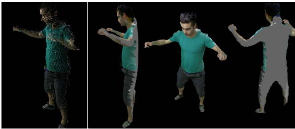
Fig. 6: Argyris sequence - Results using only two frontal captured views. Left: Raw point cloud without head. Right: Reconstruction with the head.
