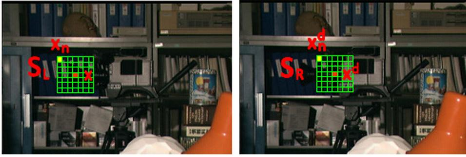
Fig. 4. Adaptive weights support region on reference and target “Tsukuba” images.
