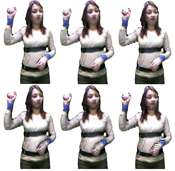
Fig. 15: Frame #615 from "Stavroula" sequence. Top row rendered without lighting and bottom row rendered with flat shading. From left to right: uncompressed mesh | proposed method at 19.8 bpvf | MPEG-4 TFAN [1] at 20.09 bpvf.
