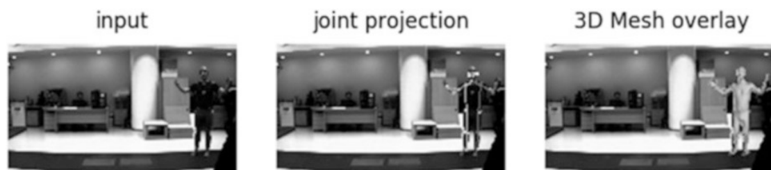
Fig. 2 Sample input frame, estimated 2D joint locations and 3D mesh overlay
