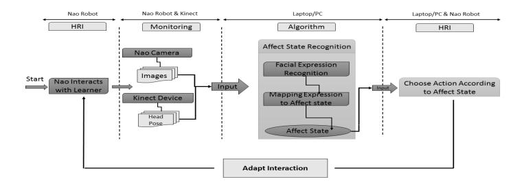
Fig. 1. A full cycle of our framework. Nao robot begins interaction with the learner, e.g. a learning task. Robot's camera and Kinect device inputs the affect recognition algorithm with images of the learner and her/his head pose respectively. The algorithm outputs the affect state of the learner and the robot decides for its next action accordingly.
