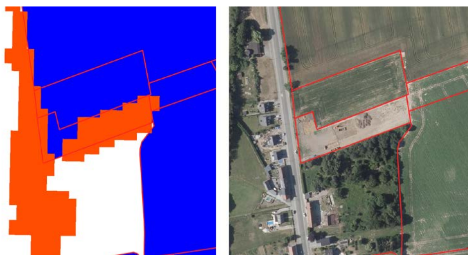
Figure 1 (left) detection of a new construction zone (right) orthophoto verification
