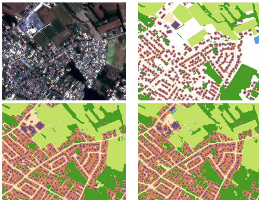
Figure From top to bottom and left to right: crop of a SPOT-6/7 image, associated reference map, classification result out of SPOT-6/7 imagery alone, classification result using both SPOT-6/7 and S2 images (dark green: forest/high vegetation ; light green: crops and low vegetation ; magenta: buildings ; grey: roads ; orange: building neighbourhood ; blue: water areas)
