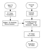
Figure 1: The watermark embedding procedure.
