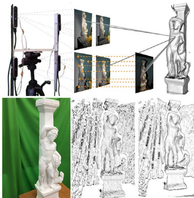
Figure 1. An abstract representation of the proposed method. Our model exploits depth-image-based rendering in a multi-view setting to achieve self-supervision using photometric consistency and geometrical and surface priors. A denoising example is visualized in the lower part (right-most), compared to a traditional filtering result (middle).
