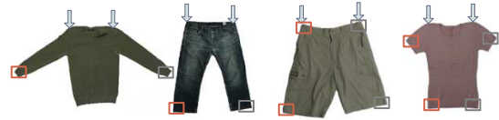
Fig. 2. Possible lowest points. Gray squares are the symmetric points of the red ones. Arrows show the desired grasping points for unfolding.
