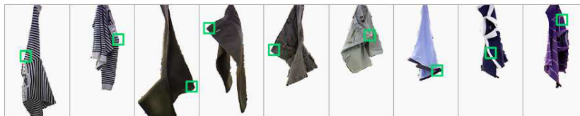
Fig. 7. Examples of successful grasp point detection
