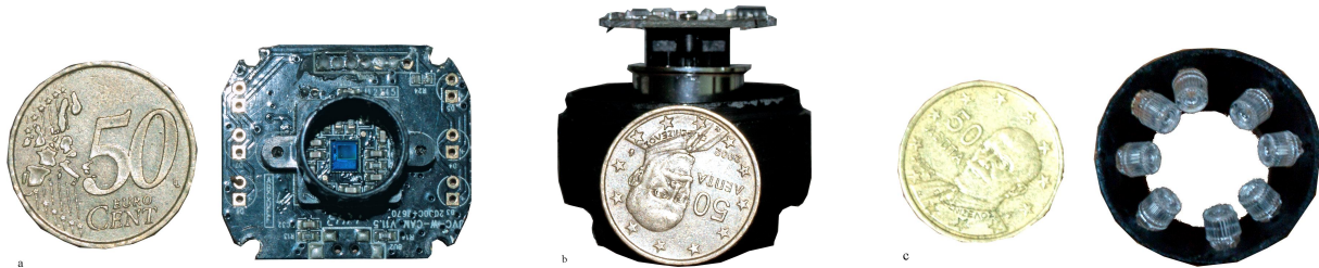
Figure 3. The camera board with rounded corners (a), the lower part of the cylindrical tube with the camera mounted (b) and the light ring (c), all compared to 50-cent euro coin.
