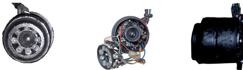
Figure 1. Front view (left), side view (right) and cross-sectional view (middle) of the lab prototype photometric stereo system.
