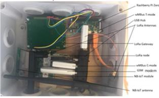
Fig. 1. Custom gateway and its electronic components
