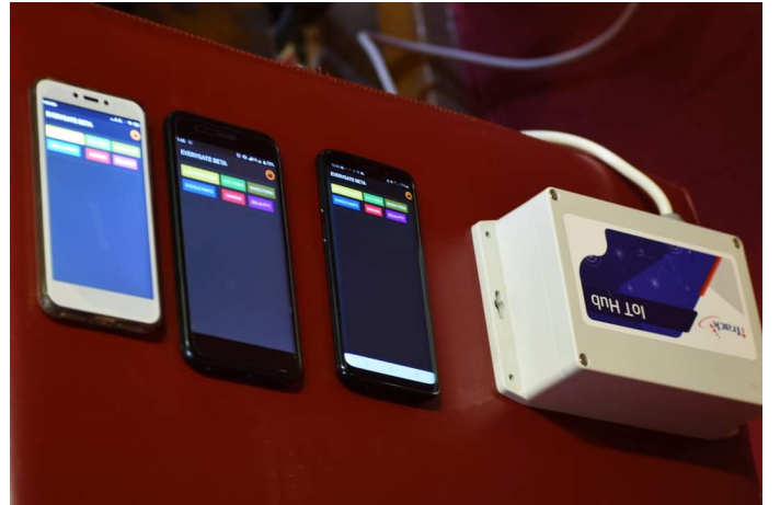
Fig. 2. Smart phones running the Everygate application collecting data from a smartband. The IoT Hub contains a smart phone and a power adaptor.
