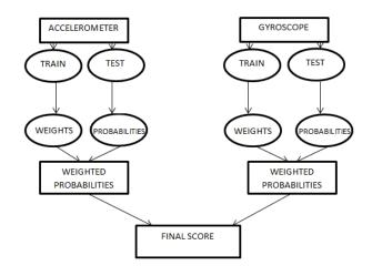
Fig. 4. Implementation of the modified class-based weighted late fusion
