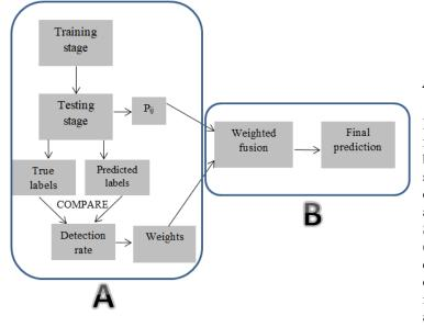
Fig. 1. Flowchart of the proposed weighted late fusion framework. Procedure in A is repeated for each sensor, while B refers to the combination of sensors.
