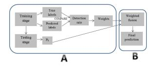
Fig. 2. Flowchart of the modified class-based weighted late fusion framework. Procedure in A is repeated for each sensor, while B refers to the combination of sensors.
