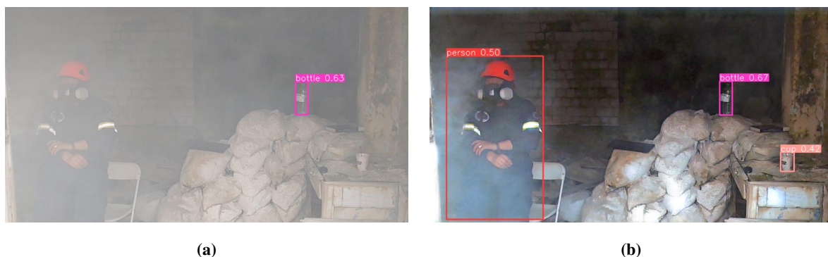
Figure 5. Object detection during the field trial in Greece: object detections (a) without desmoking and (b) after desmoking
