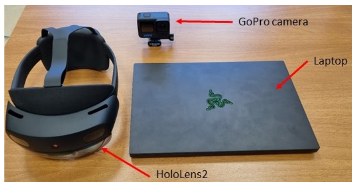
Figure 2. The main hardware components used in the proposed system: GoPro camera for image acquisition and wireless connectivity, a powerful GPU-equipped laptop for processing, and the HoloLens 2 for visualization.
