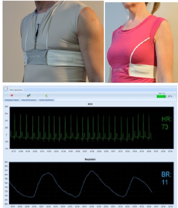
Fig. 4. On the top, an example of the textile sensing platform for man and for woman and on the bottom, an example of the ECG and Breathing Rate (BR)
