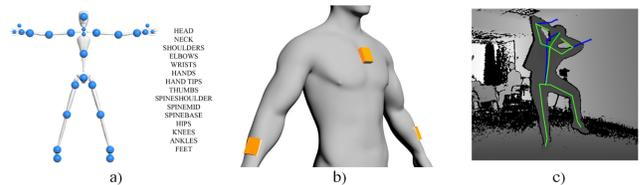
Fig. 3. a) Motion Capture structure of 25 human body joints. b) 3-WIMU body placement (on thorax and forearms). c) The blue and the green skeleton represent the Kinect Skeleton tracking and the enhanced fused skeleton estimation using Kinect/WIMUs, respectively.
