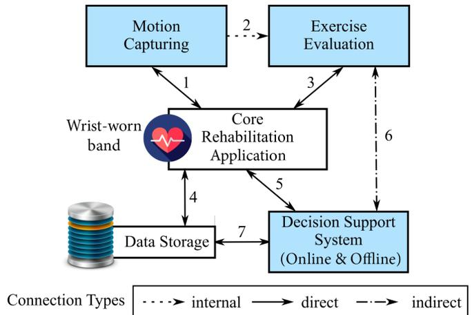
Fig. 1. High-level diagram of the module (cyan components) integrated in a rehabilitation platform.
