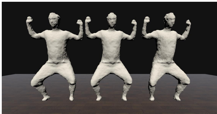
Fig. 2. Screenshot from the VR application showing the reconstructed human meshes. The reference model is in the middle while the two distorted are to its left and right.
