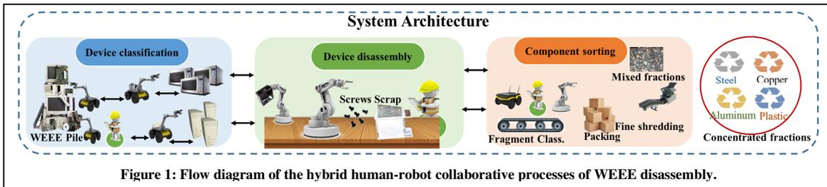
Figure 1: Flow diagram of the hybrid human-robot collaborative processes of WEEE disassembly.
