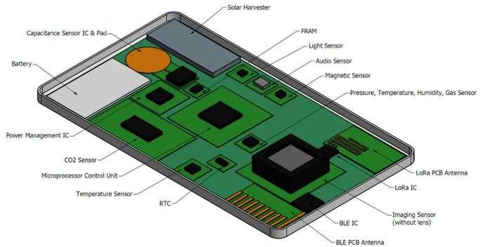
Fig. 2. Conceptual component placement on the AMANDA ASSC
