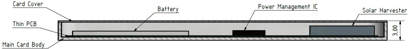
Fig. 1. Cross section of the AMANDA ASSC
