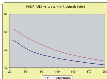
Figure 4: PSNR values for different watermark length.
