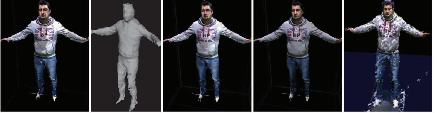
**Fig. 2.** i) Volumetric reconstruction after appropriate background subtraction (no enhancement); ii) Smoothed model without texture; iii) After weighted texture mapping; iv) After color matching; v) 5 separate meshes, reconstructed with terrain triangulation on the image plane [6].
