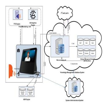
Figure 3: Flowchart of voice function subsystem and interactive models.
