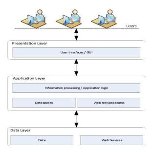
Figure 2: Three-tier Client-Server model.
