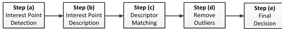
Fig. 1 Block diagram of the core analysis steps that are applied by the object re-detection algorithm of [6]
