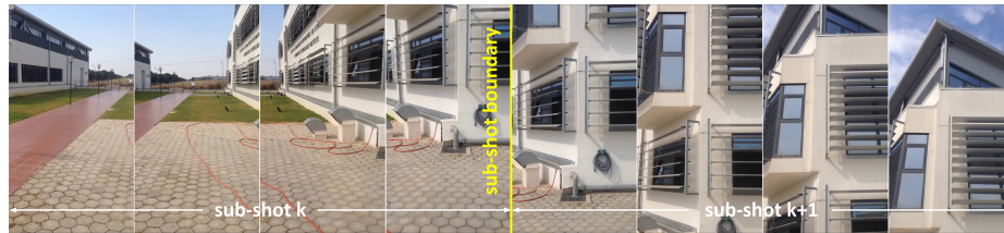
Fig. 4: A sequence of video frames (sampled for space and presentation efficiency) segmented by the proposed algorithm into two sub-shots; one related to a horizontal and one related to an upward camera movement.
