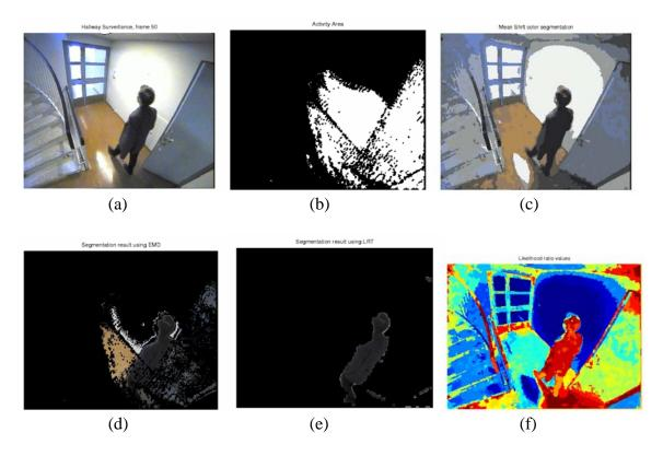
Fig. 11. Surveillance of hallway. (a) Frame 50. (b) Activity Area. (d) Mean Shift color segmentation. Segmentation results: (e) EMD, (f) LRT. g) Likelihood ratio values.
