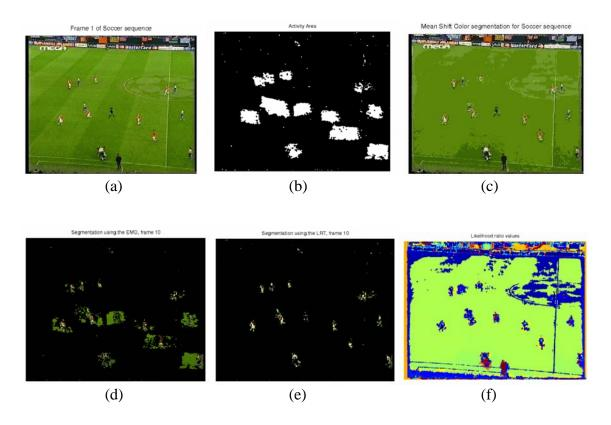
Fig. 8. Soccer Sequence. (a) Frame 1. (b) Activity Area. (c) Mean Shift color segmentation. Soccer Sequence segmentation results. (d) EMD-based for frame 10. (e) LRT-based for frame 10. (f) Likelihood ratio values.
