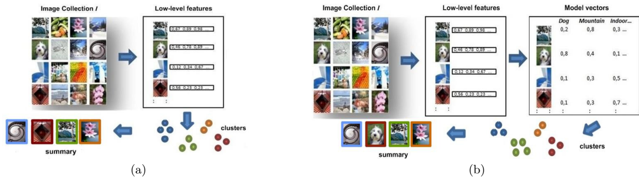
Figure 1: Clustering examples. (a) Typical image clustering approach. The clustering algorithm is applied directly to the low-level visual features. (b) Proposed concept-based clustering approach. The clustering is performed on the responses of a pool of automatic concept detectors. These detectors are not manually selected to match the contents of the image collection, and their introduction into the clustering pipeline does not require any kind of user interaction (i.e. the entire clustering process remains fully automatic).
