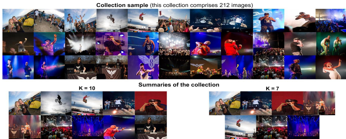
Figure 4: Summarization of an image collection of a social event produced using the model vectors in combination with the farthest first algorithm.
