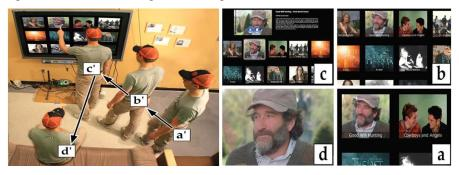
**Fig. 2.** Proxemic Interaction: a) activating the system when a person enters the room, b) continuously revealing of more content with decreasing distance of the person to the display, c) allowing explicit interaction through direct touch when person is in close distance, and d) implicitly switching to full screen view when person is taking a seat. From [23].
